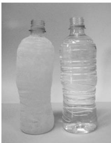
Figure 5. Expansion of water upon freezing. Water is one of the few substances that expand upon freezing. The expansion is due to the open structure of ice relative to that of liquid water.
